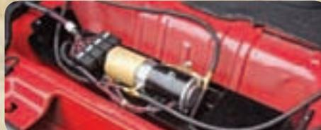
The Name Power Top comes from a durable electric power plant that has been specially developed for strength and size. This heavy duty motor installs in the storage compartment in the rear of your Jeep® keeping the rear cargo area clutter free. Each Power top includes the necessary wiring harness to make installation as easy as possible.
