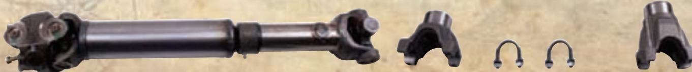
16592.21 CV Equipped Rear Drive Shaft for 07-12 Wrangler 2-Door
