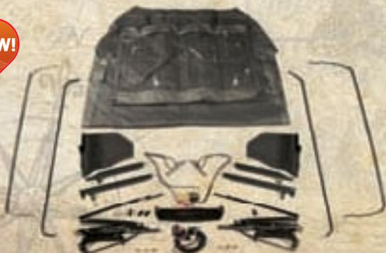
Each Power top is a complete kit that includes everything you need for installation to your 2007-2012 four door Wrangler: heavy duty sailcloth fabric, 31% tint 30 mil rear window glass, power top frame, hydraulics, motor, wiring harness and an in-depth installation packet. Bolt-on installation, No fabrication necessary.
