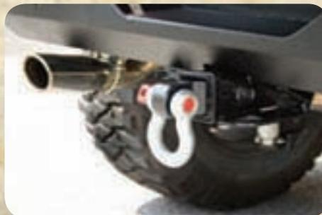
This heavy-duty steel design fits into any 2" receiver box. It is rated up to 9,500 lbs. pulling capacity on evenly distributed straight pulls. Note: never exceed your receiver capacity. Not designed for towing. Does not include hitch pin.
