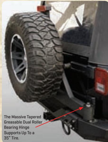
The Massive Tapered Greasable Dual Roller Bearing Hinge Supports Up To a 35" Tire.
