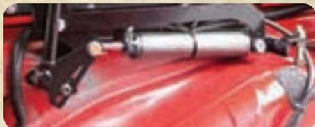
A durable hydraulic piston provides the torque to lift and retract the Power Top. Easily secured to the vehicle wheel well and soft top frame, this durable component has been cycle tested to ensure a long life and consistent performance.
