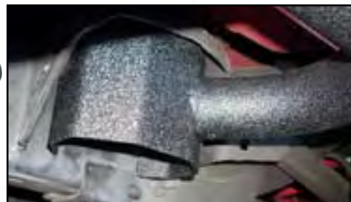
07-10 Wrangler models have simple bolt on design. Utilizes existing body mount locations on frame.
